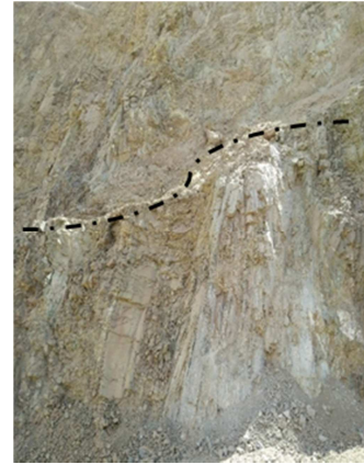
Figure 3. Fracture due to a fault in the roof.
